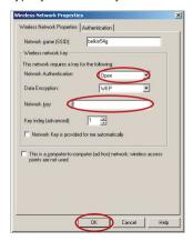
**Important:** WPA-PSK is a mixture of numbers and letters from A–Z and 0–9. For WPA-PSK you can enter eight to 63 characters. This Network key needs to match the key you assign to your Wireless Modem/Router or access point.
